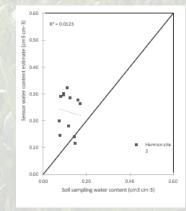
The graphs above show the relationship between water content measured via soil sampling and water content estimated by the Sentek Soil Moisture probe on the four sites studied.
